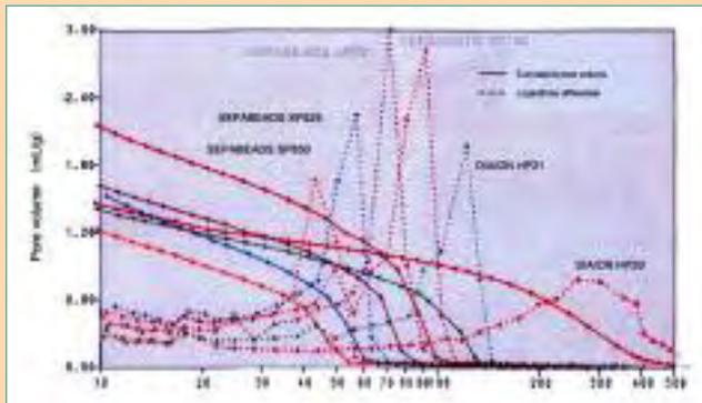
Pores distribution in adsorbent resins
